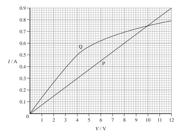
(i) State the value of the current for which the resistance of P is the same as the resistance of Q and determine this value of resistance.
