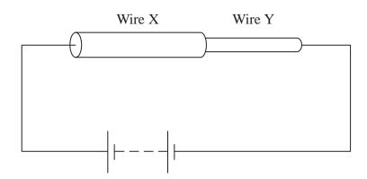
The cross-sectional area of wire X is twice the cross-sectional area of wire Y.
