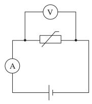
The cell has a negligible internal resistance. The effect of decreasing the temperature of the thermistor is that the
